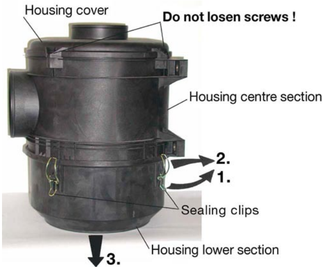
Figure 1: Removing lower housing section
