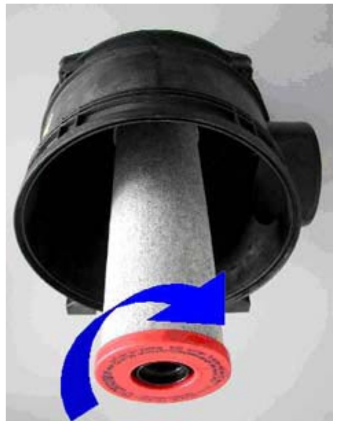
Figure 5: Installing the secondary element.
