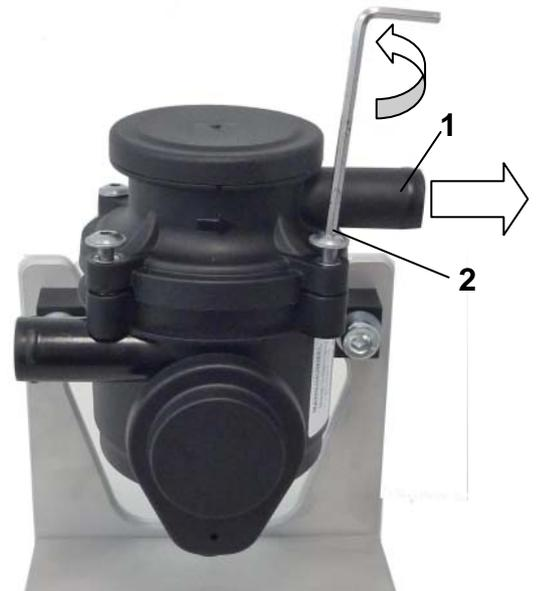
Fig. 10 Detaching lid of ProVent 100
