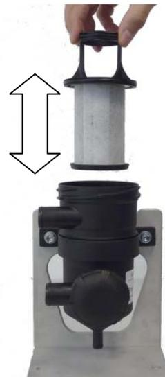
Fig. 15 Changing oil separator of ProVent 200
