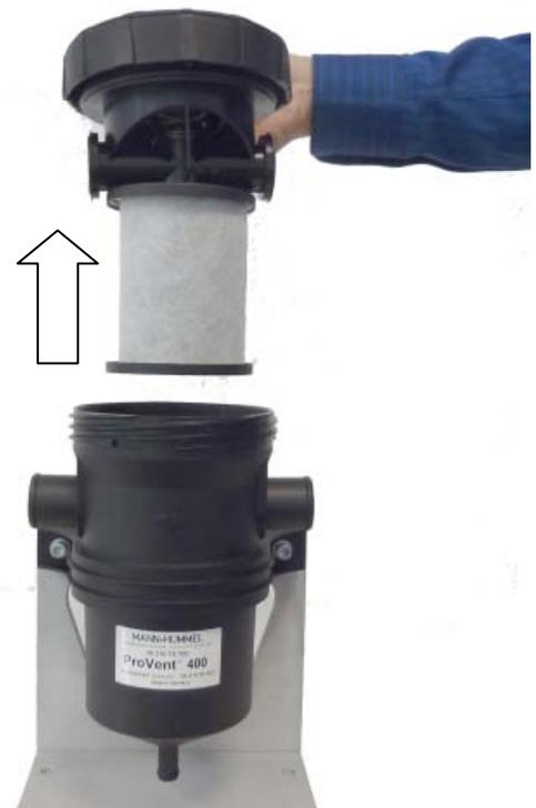
Fig. 18 Removing oil separator of ProVent 400
