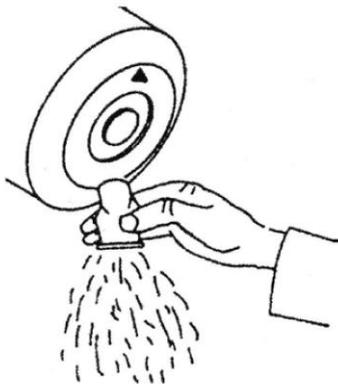
Fig. 9 Cleaning the dust discharge valve
