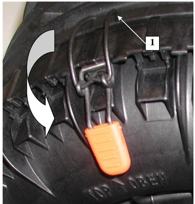
Fig. 7 Close the wire clamp fasteners
