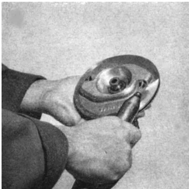
Fig. 4: Blowing out nozzles
